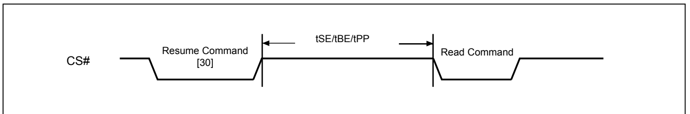
Figure 85. Resume to Read Latency
